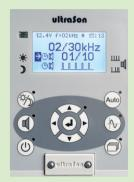
Water resistant aluminum case, 3 piezo tweeters, illuminated LCD-Display with easy to use press buttons on the back, twilight sensor, frequency regulator 2 - 30 kHz, interval and interval time regulator, night operation.
